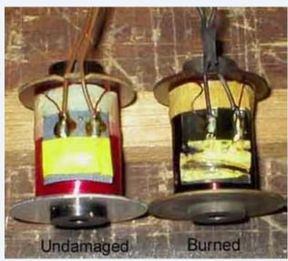
the pump won't function at all. Further, if the power is left on long enough while an all-electronic pump is stalled in a current on condition, damage will be done to the circuit board.
